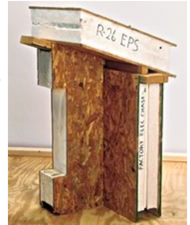
SIPs consist of an inner insulating core and two outer skins or facings. The author uses this corner and roof mock-up to demonstrate SIP connections.
